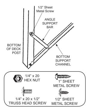
Bend the ends of the Special Bottom Support Channels and assemble as illustrated on Close-ups 7 & 8.
